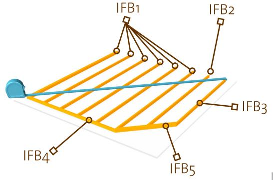
MAKE SURE THAT THE FOUNDATION IS INSTALLED ON A LEVEL SURFACE. CHECKING ALL DIRECTIONS, INCLUDING CORNER TO CORNER. 3%
