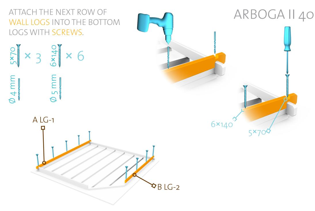
AFTER PLACING 3-4 ROWS OF WALL LOGS, TAP EACH WALL LOG IN PLACE USING A HAMMER AND THE HITBLOCK PROVIDED, TO TIGHTEN THE LOGS.
