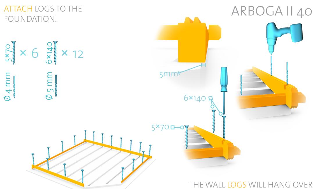
THE WALL LOGS WILL HANG OVER THE FOUNDATION BEAMS BY APPROXIMATELY 5MM. THIS OVERHANG IS DESIGNED AS A RAIN DRIP. 6%
